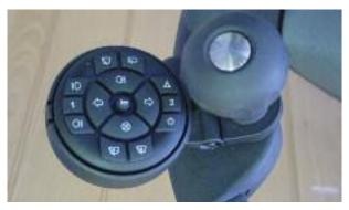
Steering knob combined with wireless secondary controls – Lodgesons
