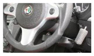
Single lever accelerator and brake – here fitted with optional indicator switch – Jeff Gosling
